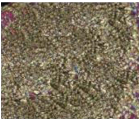
Figure 5. POM microphotograph of the polymer at 185°C.
